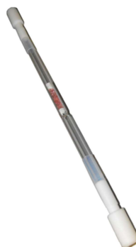
Tekran Gold-Quartz Sampling Trap
