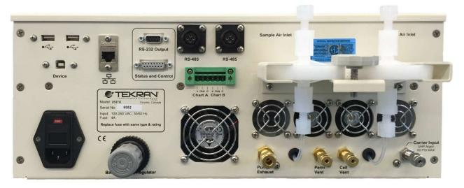
USB Host Ports (2) Network Port (1) Analog Chart Outputs (2) Status and Control Input (1) USB Device Port (1) RS-485 Ports (2) RS-232 Serial Output (1) Sample and Gas Inputs (3)
