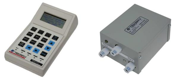
The *Tekran*<sup>®</sup> Model 1110 Synchronized Two Port Sampling System gives the Model 2537 Mercury Vapor Analyzer the ability to sample from two separate input sources. Switching between the two sources is synchronized with the instrument sampling cycle. The number of sampling cycles in each position is user programmable.
