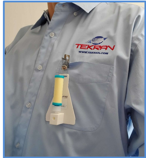
MerPAS used for worker mercury human exposure monitoring
