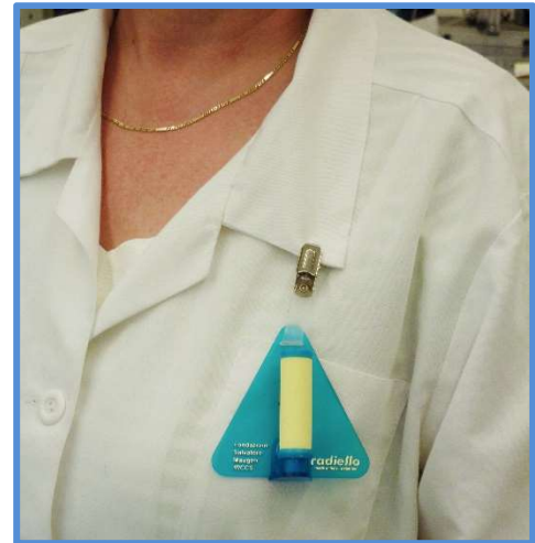
MerPAS used for worker mercury human exposure monitoring
