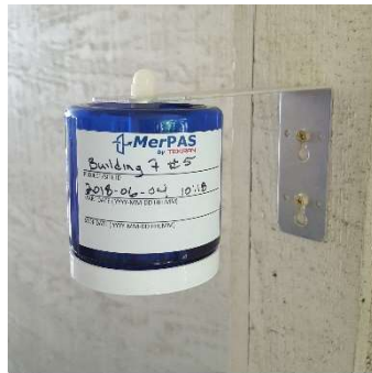
10. Proper MerPAS mounting
