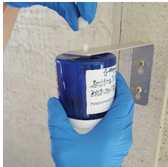
9. Attach jar to bracket
