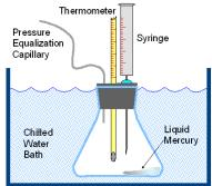
• The entry of heat through the body of standard glass thermometers can severely impact the measured vapor temperature reading. Many implementations only measure the temperature of the water bath, causing inaccuracy due to heat entry through the top of the flask.
