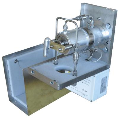
The electrically heated Tekran 3443 dilution probe is used in conjunction with the Tekran 3400 HgCEM System, where the measuring of process gas requires dilution and transport of sample gas to the detection system. The Tekran 3443 probe and filter are specifically designed for dilution and then quantitative transport of flue gases to the 3400 HgCEM conditioner . The Tekran 3443 dilution probe enables the user to adapt the probe to a wide range of sampling applications.
