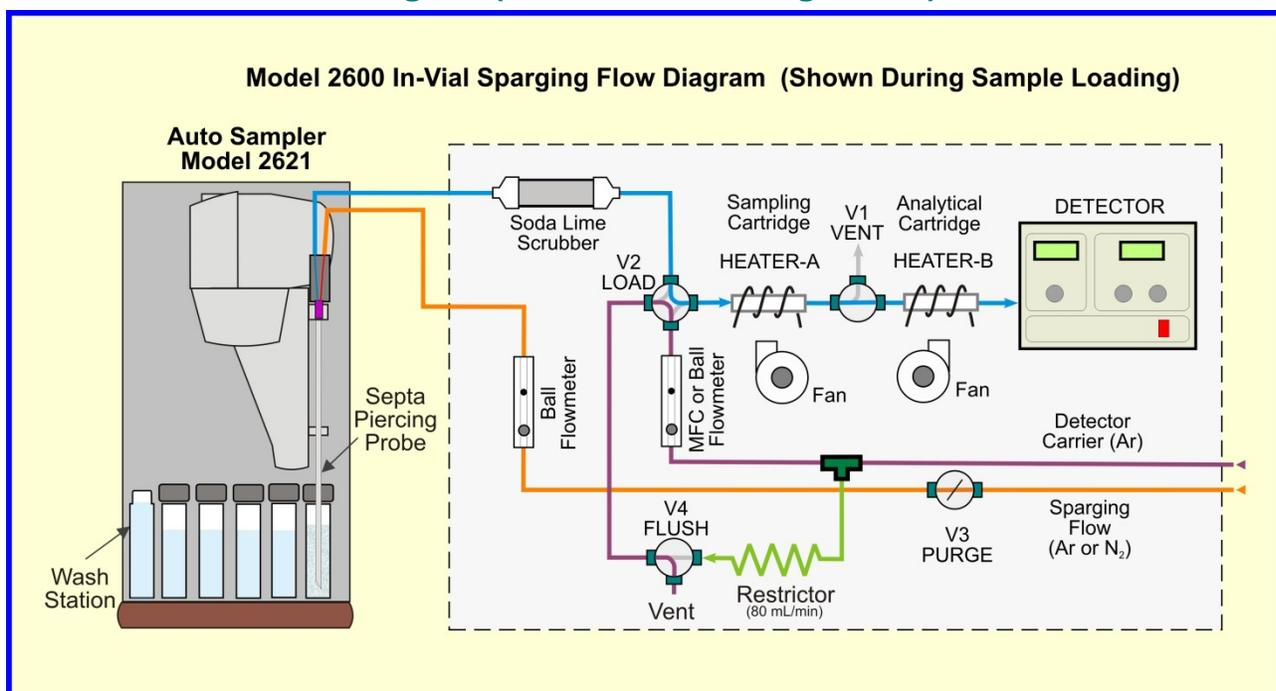
Configuring the Tekran 2600 for in-vial sparging requires installation of additional hardware such as solenoid valve, capillary restrictor, and septa piercing probe. Refer to the Tekran 2600-IVS Flow Diagram directly above. Demonstrating the adaptability of the Tekran 2600 software, the new in-vial technique is fully automated and controlled by the Tek-MDS 2.5 software package. No software update is required.
