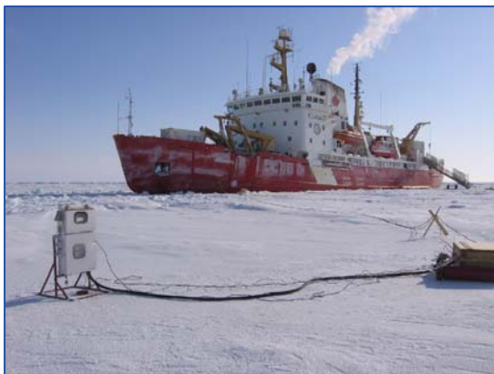
Arctic Research Vessel, Amundsen, with Tekran 2537 Ambient Mercury Speciation System in the Foreground.
